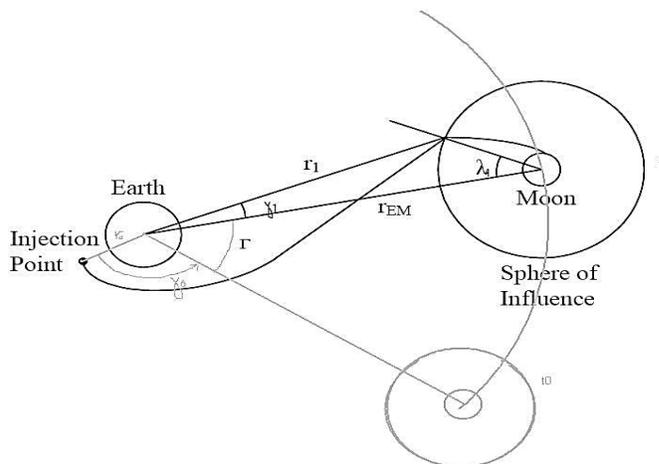
Fig 6: Patched Conic Approximation Method
