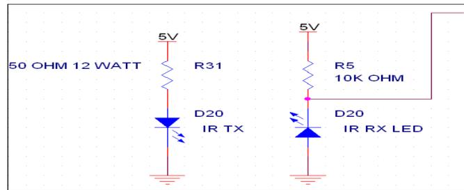
Figure 5. IR based obstacle sensor
