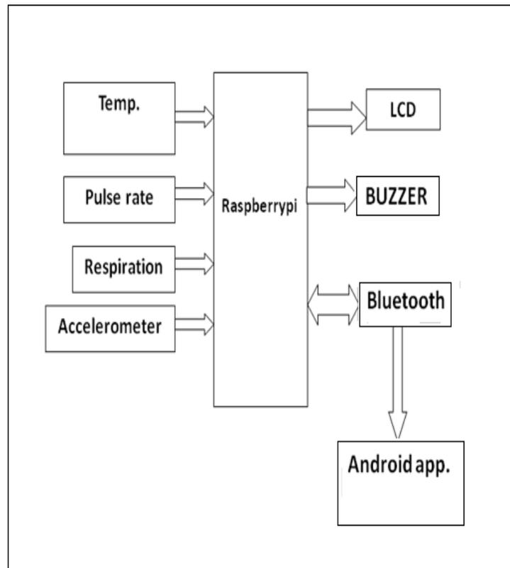
Figure 1 Block diagram of smart health monitoring system using raspberry pi
