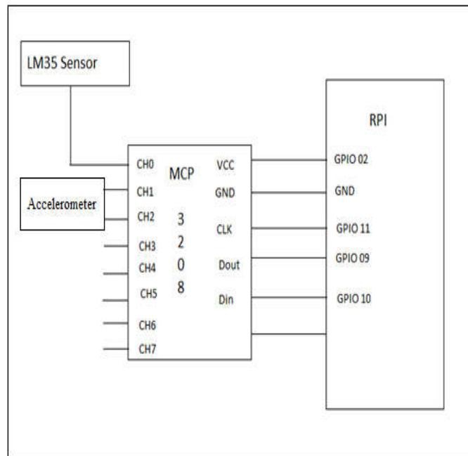
Figure4. Temperature and accelerometer sensors are interfacing with Raspberry Pi
