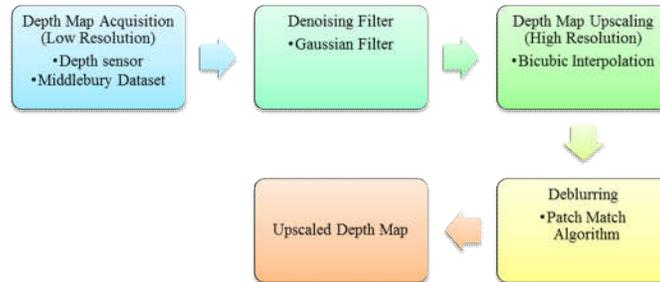
Fig. 10: Block Diagram of the Proposed System.
