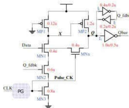
Fig (e) Modified circuit
