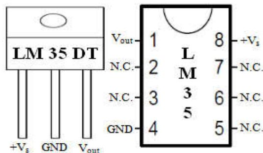
Fig. 4. Temperature sensor LM 35 DT and its pin detail.
